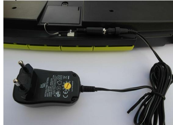
Finally connect the power supply to the socket on the Battery Supply Adapter. Take care not to overload the thin cable of the Battery Supply Adapter later on.
