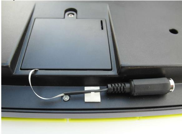
Now place the cable as you like and carefully close the battery compartment. Take care not to bend the cable – a small radius of down to approx. 1 mm is allowed.
