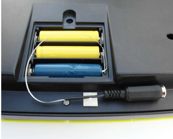
Insert the Power Supply Adapter (blue) into a suitable battery compartment **and make sure that the polarity is correct:**
